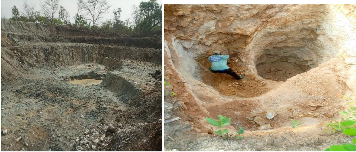
Plate 2: Open Pit: Stripping the overburden on the Spodumene (Li 2 O) Deposit
